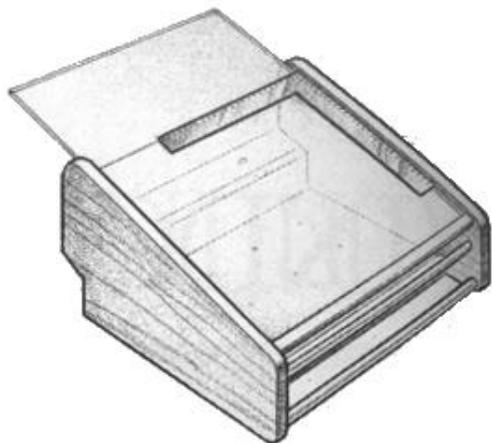
Rip acrylic panel to width, then slide into grooves and mark for length. Cut, then remove protective plastic from acrylic panel.
